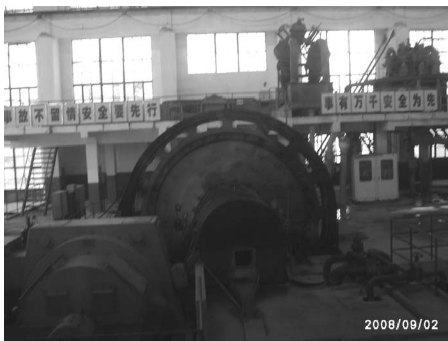
Figure 3.19: Dayukou — Phosphate Plant Hardinge Ball Mill
