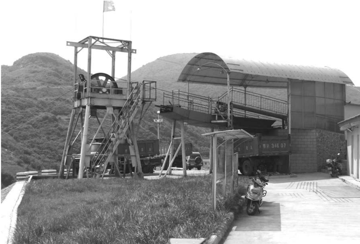
Figure 2.2: Wangji — Hoist and 8t Truck
