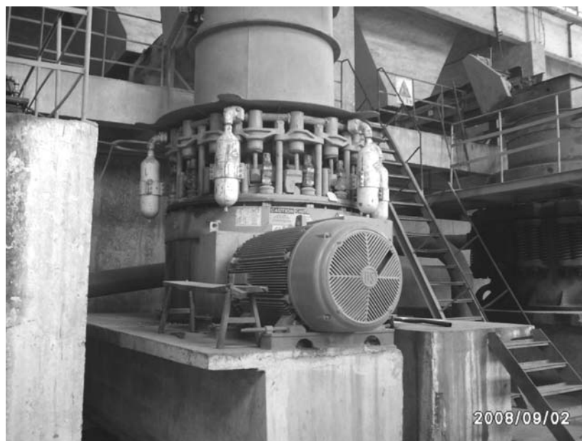
Figure 3.17: Dayukou — Phosphate Plant Tertiary Cone Crusher
